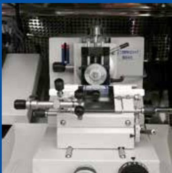
Designed to make full use of the attributes of a Feather™ blade, the Quick Release Feather™ Blade Holder enables the Cryotomist to use the full length of the blade without waste. Other important features are the fact that the blade angle can be changed without changing the position of the blade
