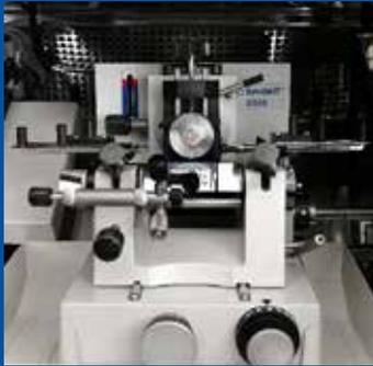
The Bright 5040 microtome is based on original and proven designs that can cope with high cutting loads and yet perform very favourably under conditions of low temperature. Based on the principle of a parallelogram of forces, the 5040 is of unique
